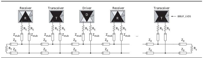
*Figure 3-22* • **BLVDS/M-LVDS Multipoint Application Using LVDS I/O Buffers**
