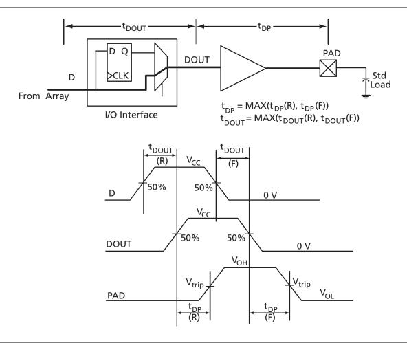
Figure 3-4 • Output Buffer Model and Delays (example)
