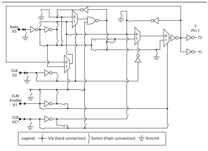
*Note:* \*This input can only be connected to the global clock distribution network. Figure 2-3 • **ProASIC3E Core VersaTile**
