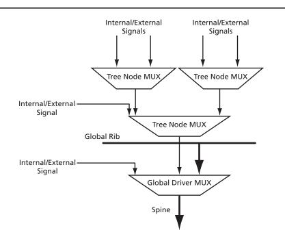
Figure 2-11 • Spine Selection MUX of Global Tree
