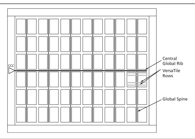
Figure 3-37 • Example of Global Tree Use in an A3PE600 Device for Clock Routing
