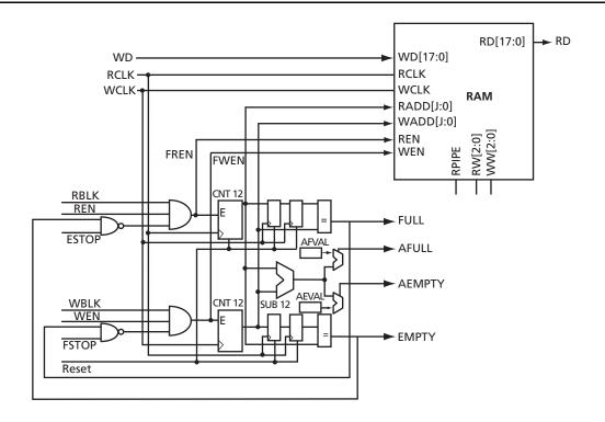
Figure 2-21 • ProASIC3E RAM Block with Embedded FIFO Controller
