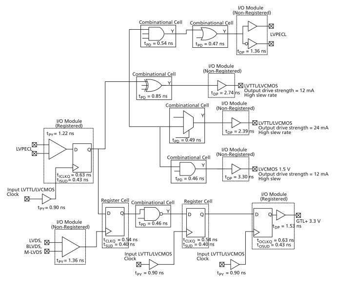
*Figure 3-2* • Timing Model Operating Conditions: –2 Speed, Commercial Temperature Range (T<sub>J</sub> = 70°C), Worst-Case V<sub>CC</sub> = 1.425 V
