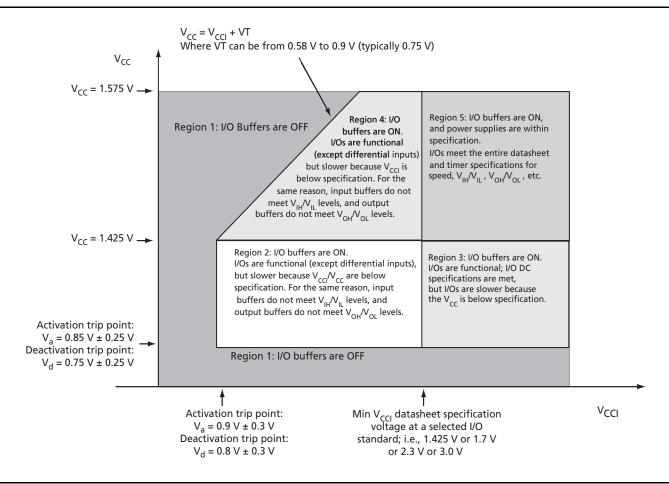
Figure 3-1 • I/O State as a Function of V<sub>CCI</sub> and V<sub>CC</sub> Voltage Levels
