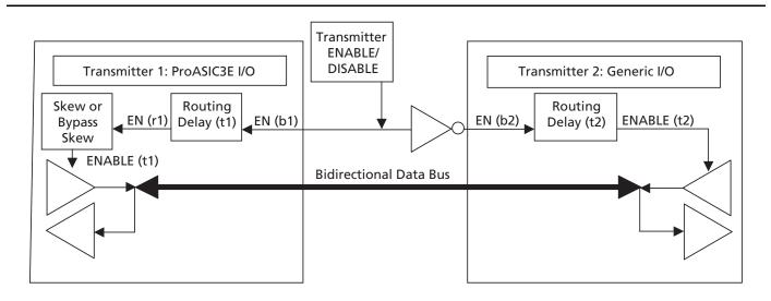
Figure 2-33 • Example of Implementation of Skew Circuits in Bidirectional Transmission Systems Using ProASIC3E Devices
