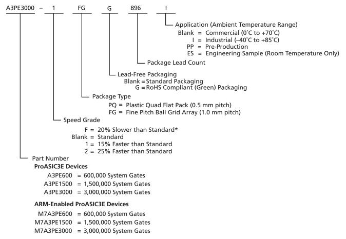
**Note:** \*–F Speed Grade – DC and switching based only on simulation. The characteristics are subject to change after establishing FPGA specifications. Some restrictions might be added and will be reflected in future revisions of this document. This speed grade is only supported in commercial temperature range.
