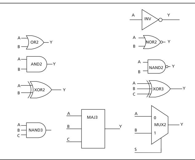
Figure 3-33 • Sample of Combinatorial Cells
