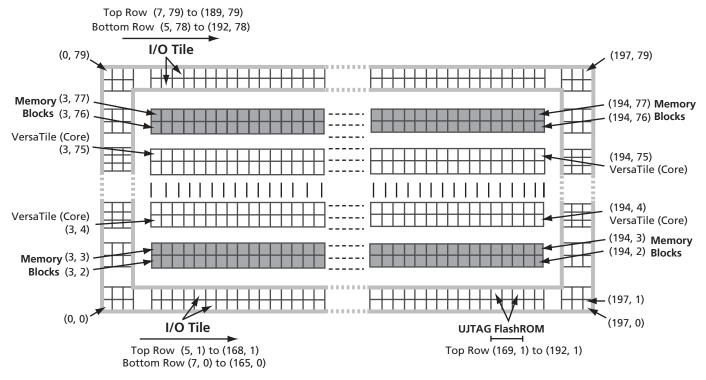
**Note:** The vertical I/O tile coordinates are not shown. West side coordinates are {(0, 2) to (2, 2)} to {(0, 77) to (2, 77)}; east side coordinates are {(195, 2) to (197, 2)} to {(195, 77) to (197, 77)}.
