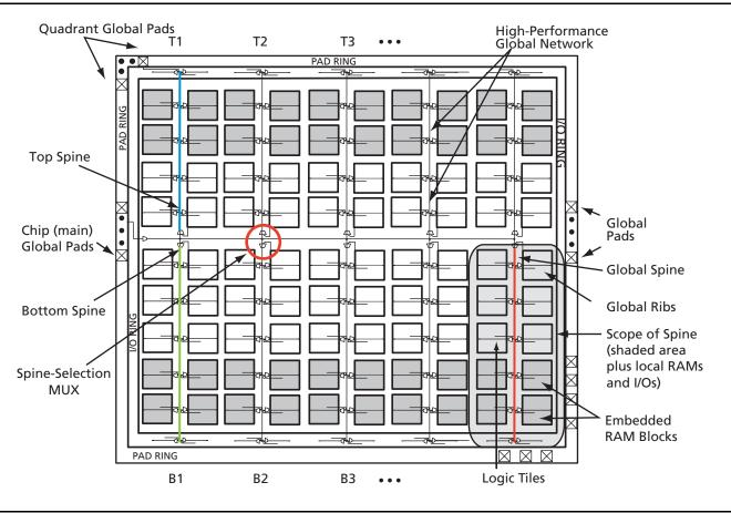
*Figure 2-10* • Spines in a Global Clock Tree Network
