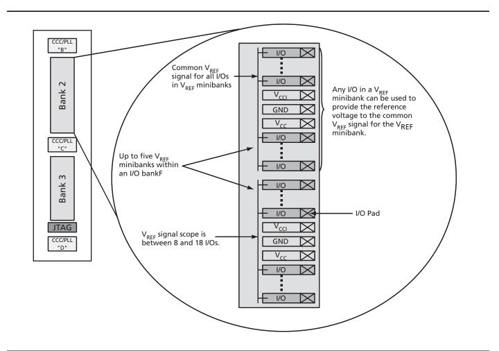
Figure 2-22 • Typical I/O Bank Detail Showing V<sub>REF</sub> Minibanks
