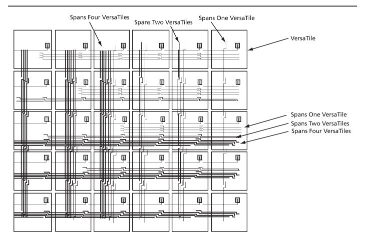
*Figure 2-6* • Efficient Long-Line Resources
