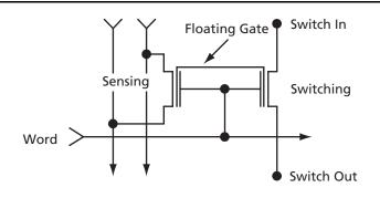
Figure 2-1 • ProASIC3E Flash-Based Switch
