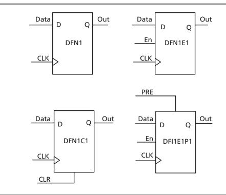
Figure 3-35 • Sample of Sequential Cells
