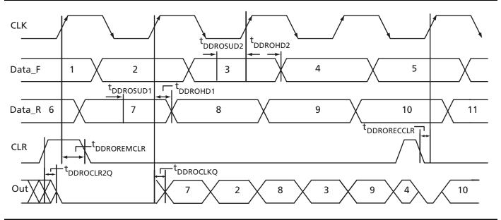
Figure 3-32 • Output DDR Timing Diagram
