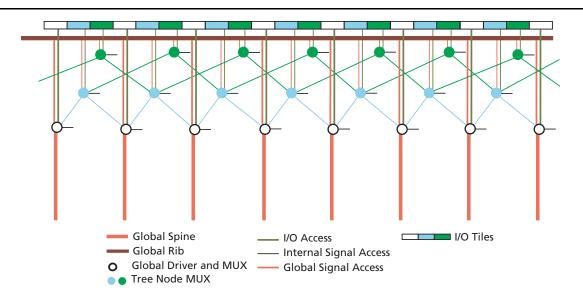
Figure 2-12 • Clock Aggregation Tree Architecture
