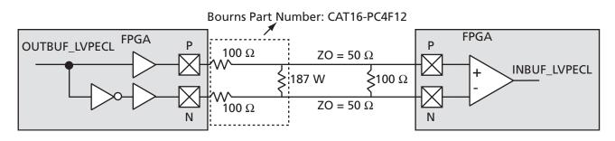
*Figure 3-23* • LVPECL Circuit Diagram and Board-Level Implementation
