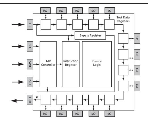
Figure 2-37 • Boundary Scan Chain in ProASIC3E
