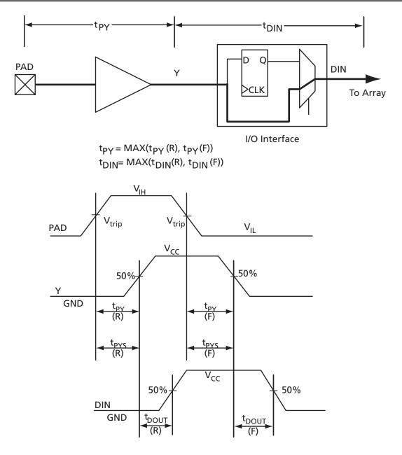
Figure 3-3 • Input Buffer Timing Model and Delays (example)
