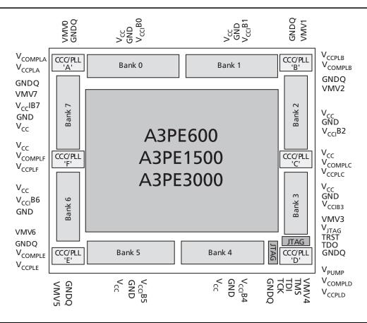
Figure 2-36 • User I/O Naming Conventions of ProASIC3E Devices
