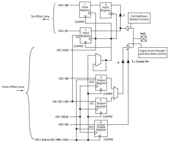
Note: ProASIC3E I/Os have registers to support DDR functionality (see the "Double Data Rate (DDR) Support" section on page 2-34 for more information).
