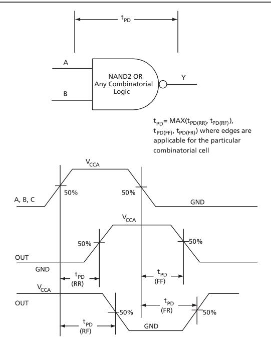
Figure 3-34 • Timing Model and Waveforms
