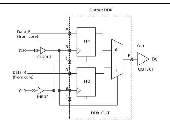
Figure 2-25 • DDR Output Support in ProASIC3E Devices
