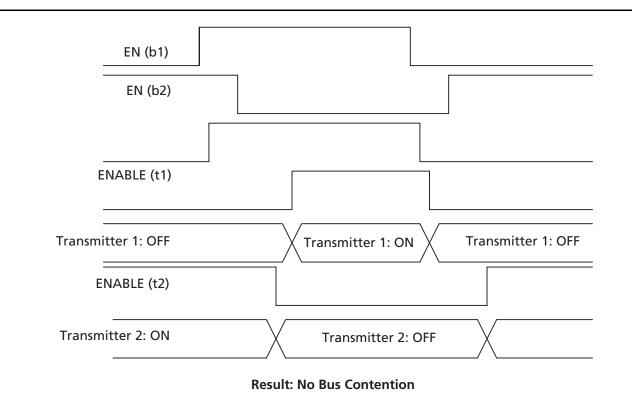
Figure 2-35 • Timing Diagram (with Skew Circuit Selected)
